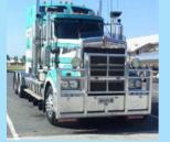
2005 MODEL, CAT C-15, 18 SPEED ROAD RANGER, DIFF RATIO 4.33 ON 8 BAG SUSPENSION, REAR MOUNT VIESA, DG SPEC HYDRAULICS FITTED.
