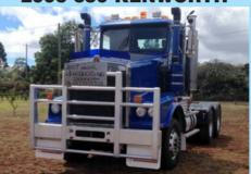
Gen 2 cummins, 18spd Road Ranger on 6 rod, PTO/HYD. Genuine 380,000km, 90T rated will rate to 120 tonne.
