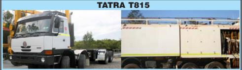
CAB & CHASSIS, OR, WITH SERVICE BODY TO SUIT. 8X8 ALL TERRAIN, LONG WHEEL BASE YEAR 06, FIT 9.7 METER BODY, INDEPENDENT SUSPENSION ALL WHEELS, ALSO CAN SELECT POSITIVE DRIVE TO ALL WHEELS, SUIT MANY APPLICATIONS, ON OR OFF ROAD, EXCELLENT CONDITION, ONLY TRAVELED 9000 KM.
