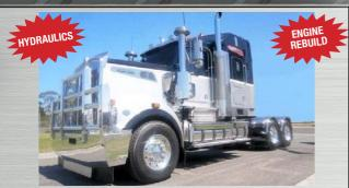
CAT @ 550HP, 18 SPD R/R GEARBOX, RT46-160 DIFFS, AIRGLIDE 460 SUSP @ 97T, ABS OFFSETS, FUPS BULLBAR, DUAL 6" STACKS, CUSTOM PAINT AND LIGHT BAR, 50" AERODYNE SLEEPER W/ COOLER
