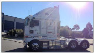
ISX Cummins @580 18 Speed 46's air glide suspension ox blood interior Double bunks viessa evaporative cooler alloy wheels FUPS ABS Deck plates electric windows and mirrors stainless everywhere. Just come into stock. Just had wheels bearings and brakes. NSW B-double registration till October this year.
